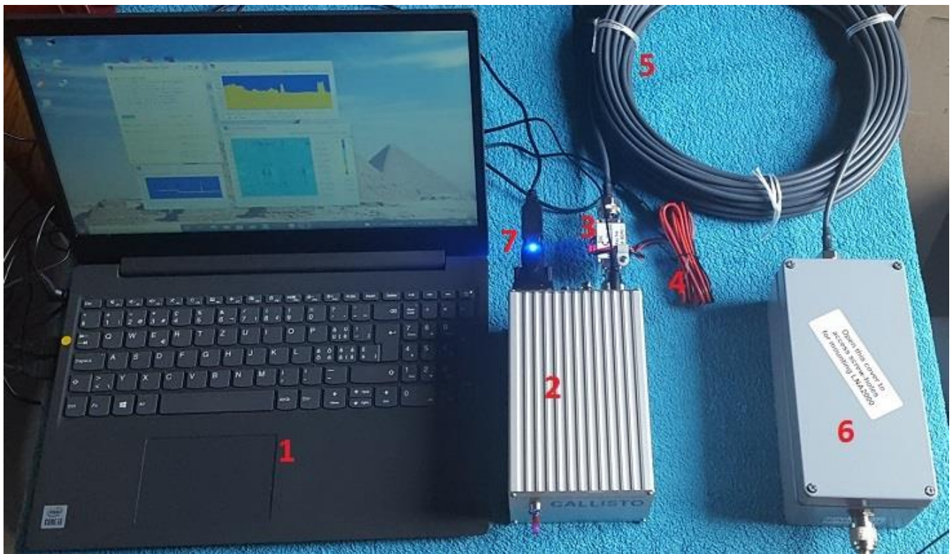
Fig. 1: Final test of equipment which was delivered to EgSA. 1=notebook, 2=Callisto, 3=Bias-Tee, 4=dc-cable, 5=coaxial cable and 6=LNA2000 with lightning protection.
