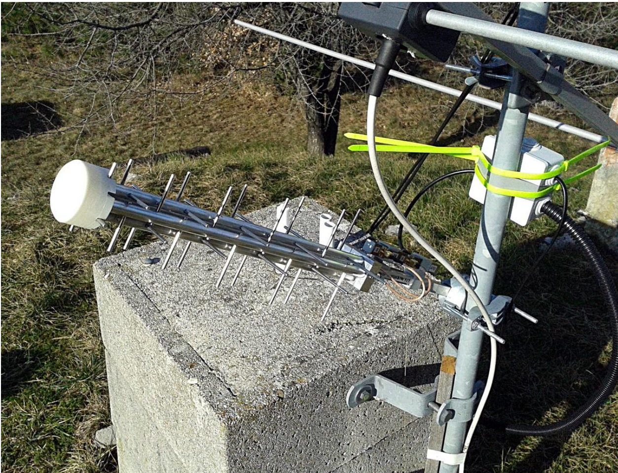
Fig. 8: Detail of L-band antenna 1.0 - 1.6 GHz (LPDA).
