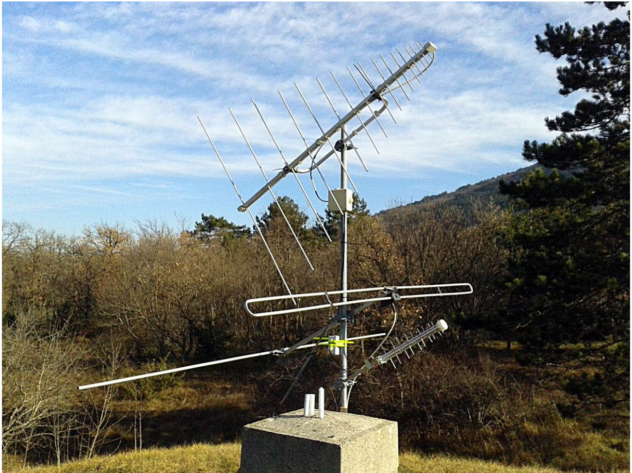
Fig. 7: Antenna farm with new L-band antenna to observe 1.0-1.6 GHz
