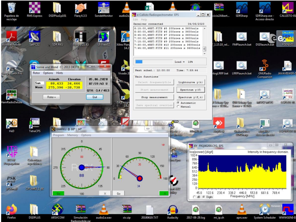
Fig. 5: Control monitor with Callisto application and rotor control application.
