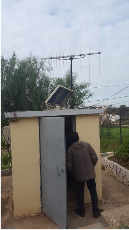
Fig. 1: Concrete shed, containing the seismometers, seismometer transmitter and PV-controller with battery. On the roof we see the antenna CLP-5130 in vertical polarization as well as the PV-panel oriented to the high noon transit of the Sun.
