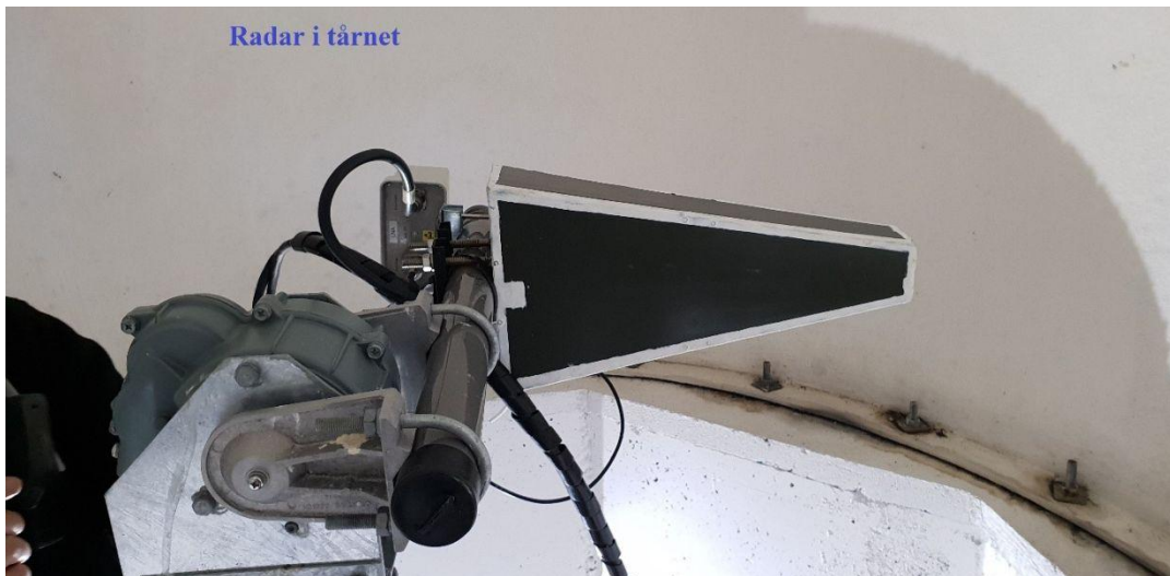
Fig. 11: Antenna (small LPDA) with protection cover and antenna mounting.
