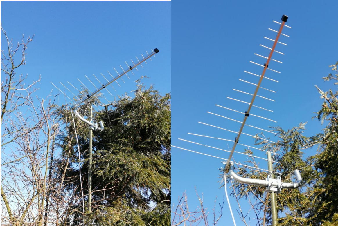
Fig. 7-8: LPDA and mounting at Hildesheim observatory, Germany
