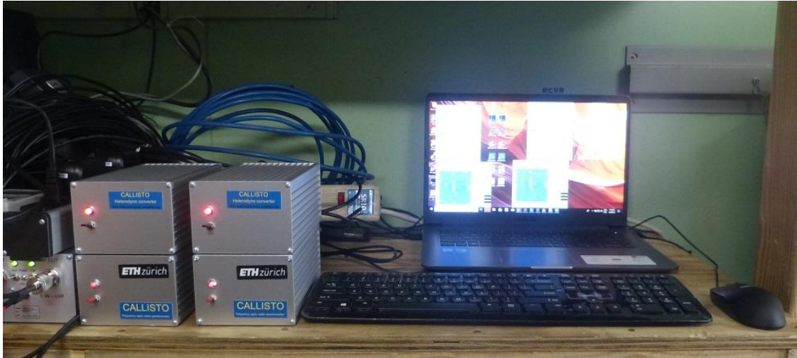
Fig. 19: Two Callisto and two heterodyne up-converter for dual circular polarization spectrometer.
