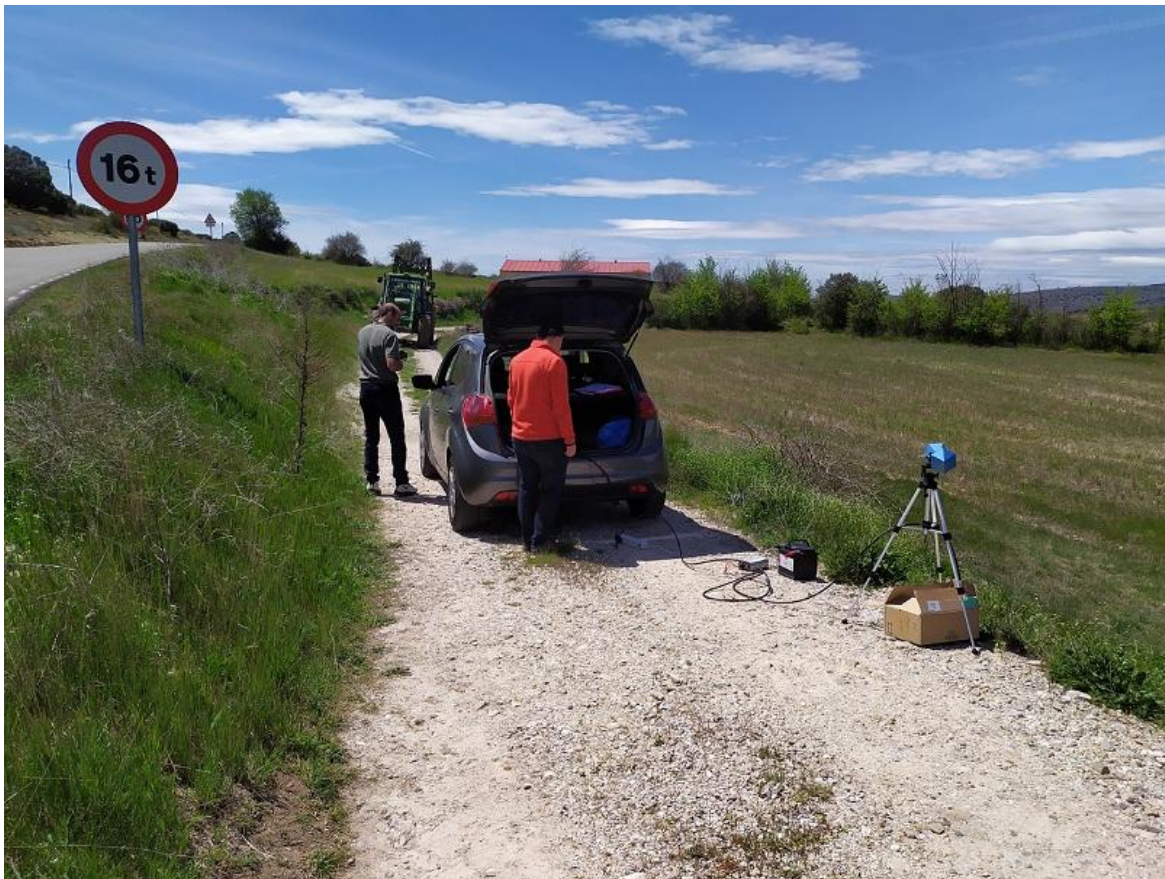
Fig. 21: Manuel Prieto Mateo and colleague repeating spectral measurements with Bicone and Callisto.
