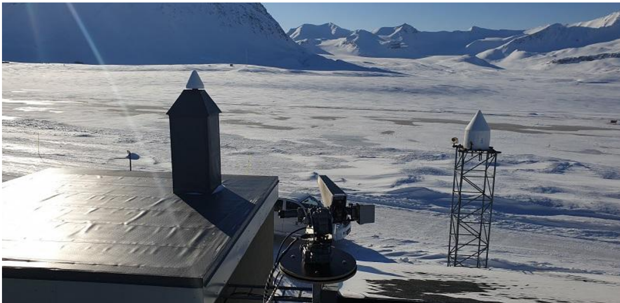
Fig. 14: LPDA on top of the mounting system.
