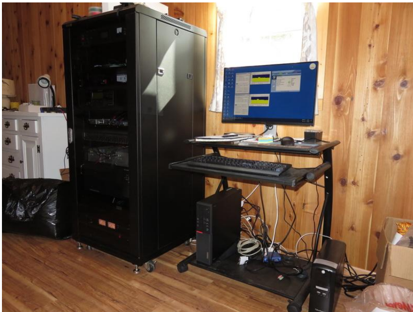
Fig. 10: Rack containing two receivers, spectrometers for circular polarization measurements, UPS and associated hardware.
