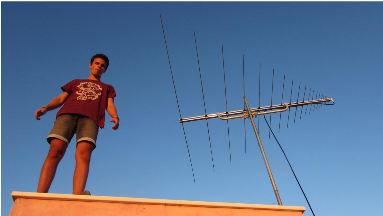
Fig. 7: LPDA antenna in horizontal polarization, pointing south (roughly). No tracking system available yet.
