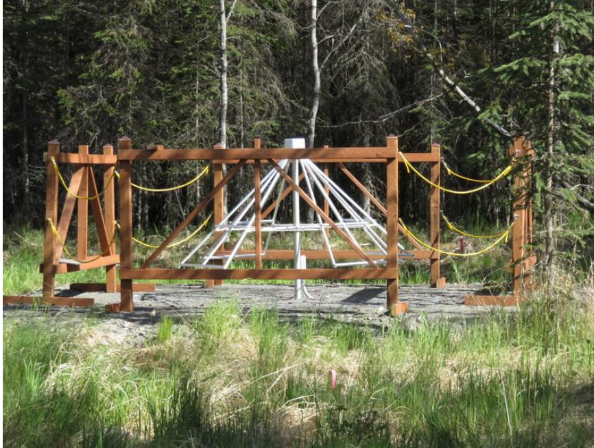
Fig. 9: Long wave antenna (LWA) in a wooden shed as protection from aggressive moose.
