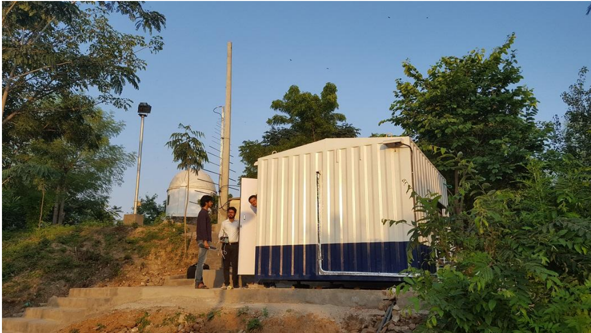
Fig. 2: LPDA mounted in the background, metallic container hosting Callisto and PC in front. The container is equipped with UPS to keep instruments working even during power outages. And the system has also an air conditioning system (a/c) to guarantee constant stability of the spectrometer.
