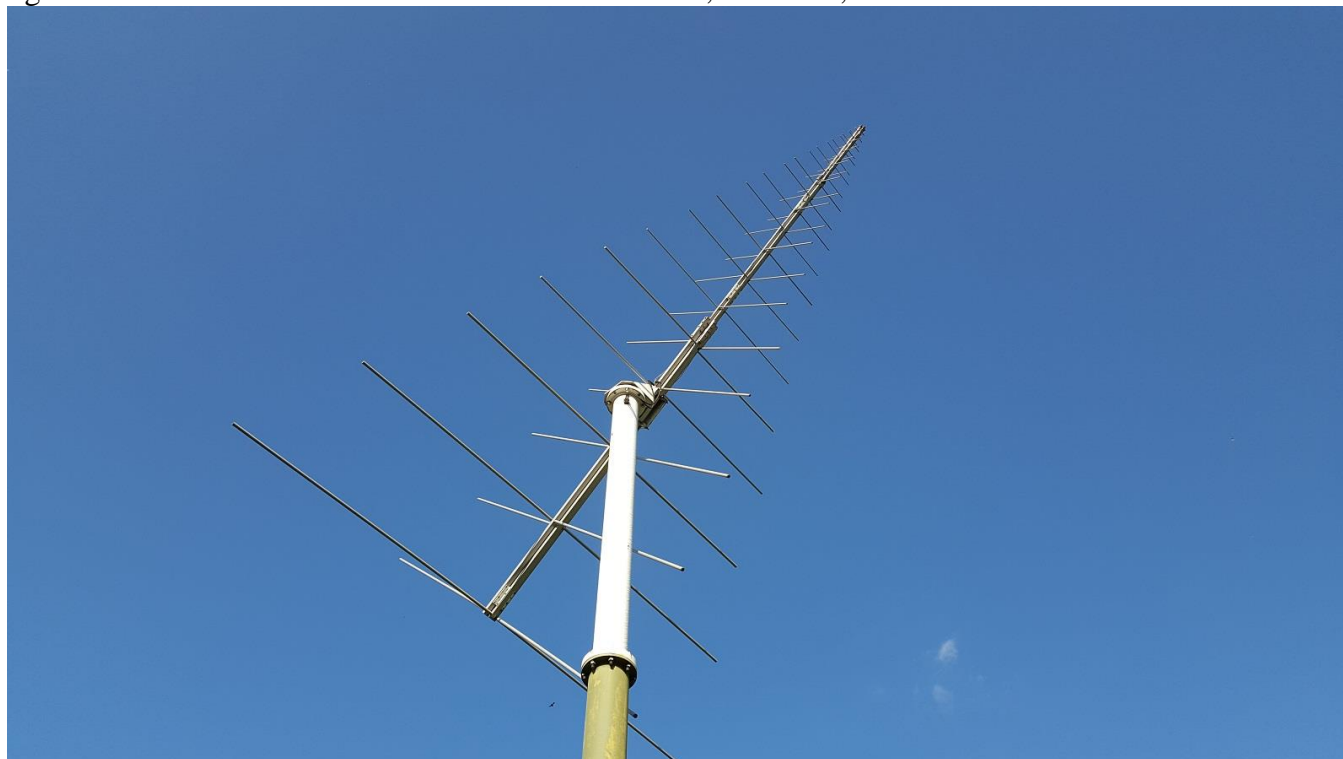
Fig 1: Dual polarization LPDA at fixed sky position to observe the Sun during transit.
