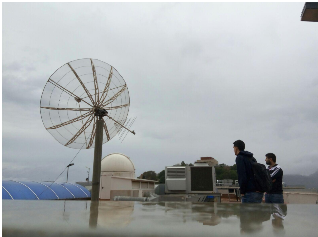
Fig. 5: Report by José Gomez: We are setting up Callisto, and one of our students, Javier Díaz is in charge of this. Above a picture of the logperiodic antenna (LPDA) installed together with the parabolic dish to use the same positioning / tracking system.
