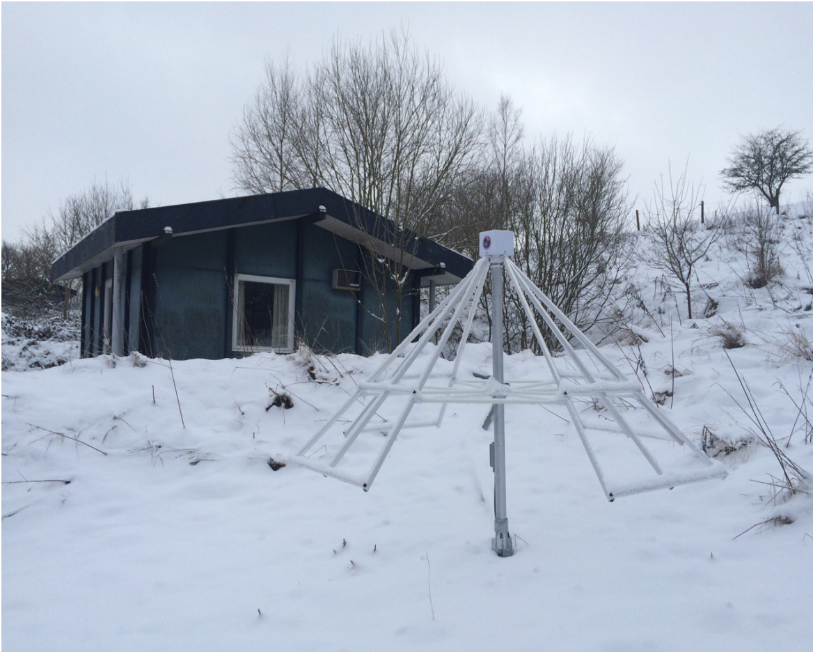
Fig. 1: LWA installed at an existing observatory site of the university. Frequency range 45 MHz – 100 MHz
