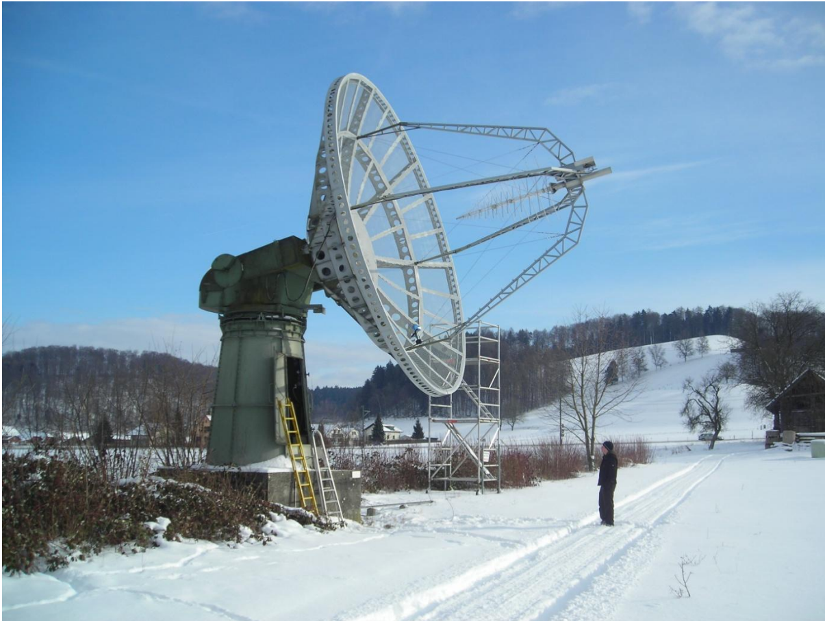
Fig. 5 ~ Parabolic dish 7 m diameter for observing from 100 MHz up to 4000 MHz in dual circular polarization at Bleien Observatory. On April 22th, 2015 solar observations have been switched off.
