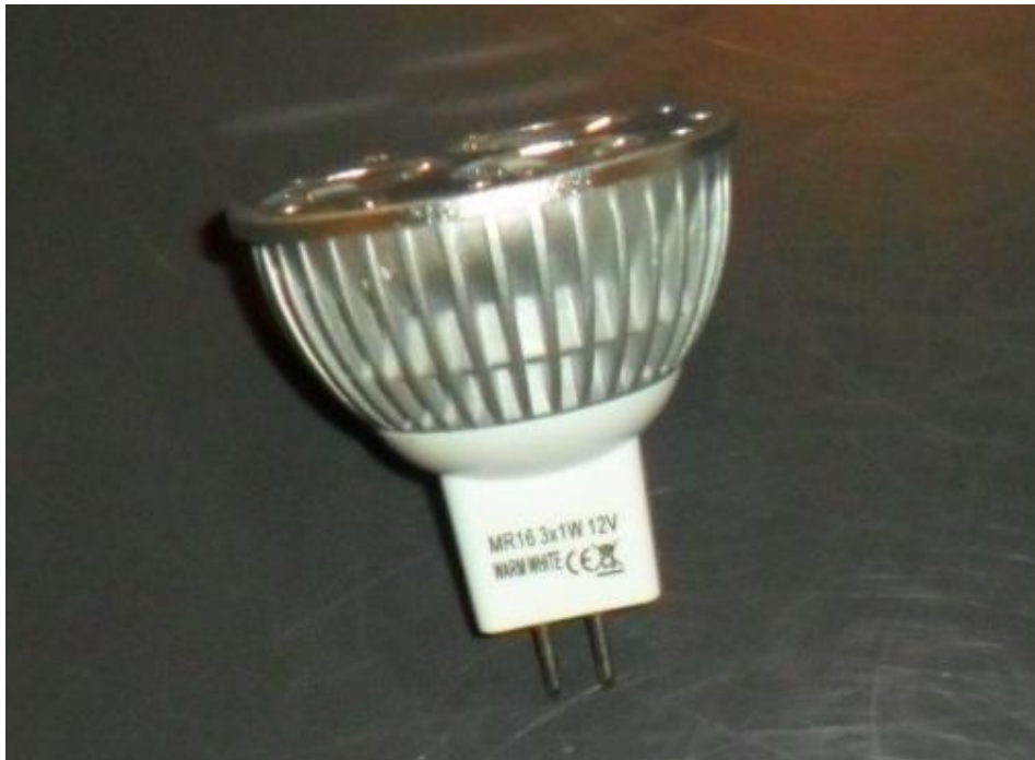
Fig. 13 ~ Guilty LED of type MR16 3*1W 12V WARM WHITE (CE), procured from LED.CH for CHF 28.60 per unit. The LED was parallel to a few other incandescent lamps and was driven by a 12V ac-transformer.
