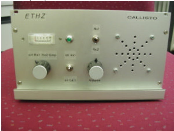
Front side of CALLISTO QM cartridge. An enclosure has not yet been defined, we are thinking about a table housing or a 19'-rack housing [TBD].
