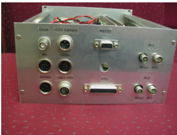
Back side of CALLISTO QM cartridge. All chassis plugs are different from each other to not confuse with all cable plugs. The hole in the center of the backplane has erroneously been made. No reason for a non-conformance report but it will be repaired in the coming FM modules.
