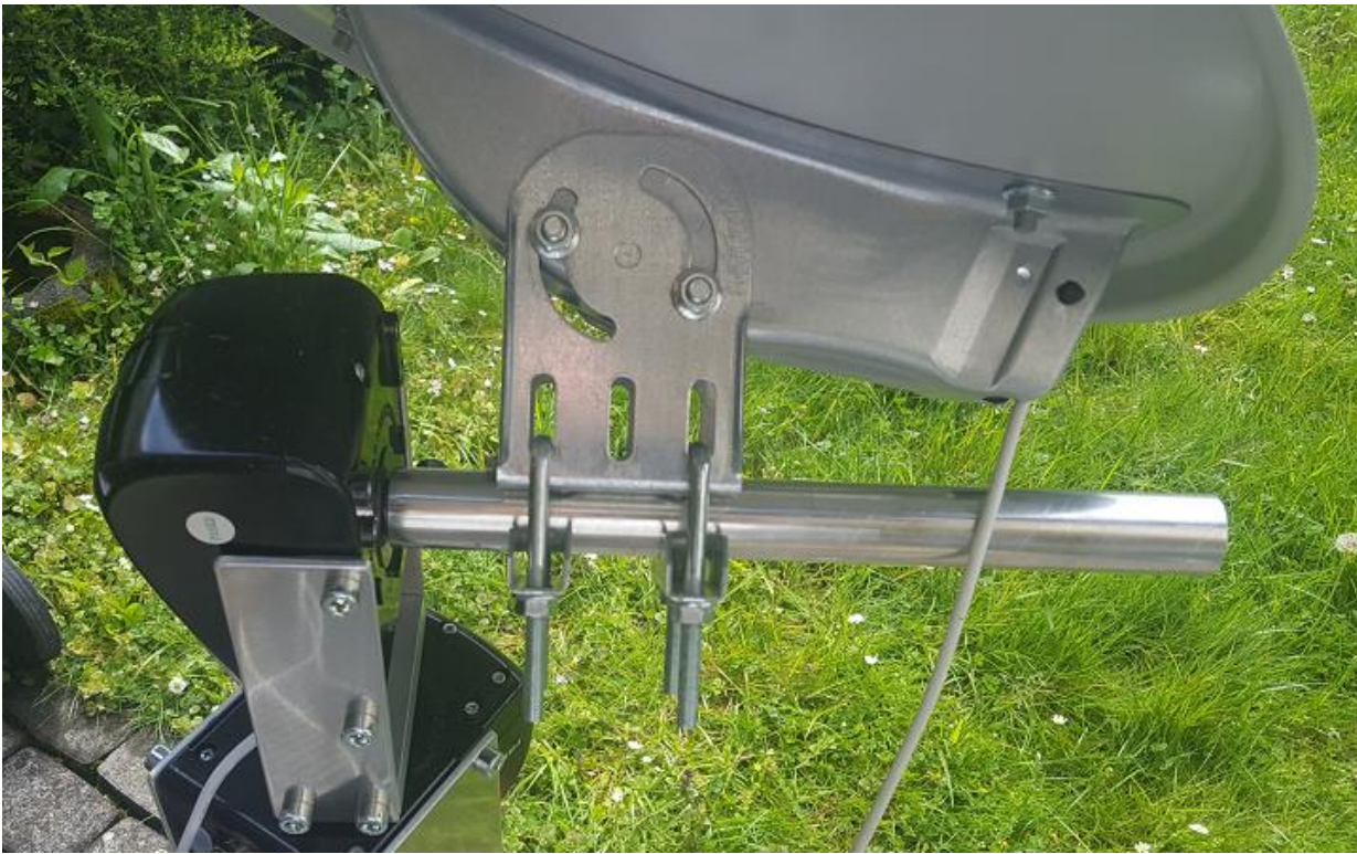
Figure 5 ~ Install antenna clamping adapter as close as possible to the elevation rotor to minimize moment on the elevation axis. While the axis is pointing west, mount dish such that feed arm and coaxial cable are also on the west side. Tighten the 4 hex-nuts with a wrench.
