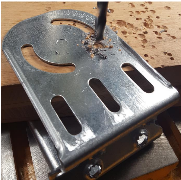
Figures 4a, b ~ Circular slits for antenna mounting need to be extended by about 10 mm, such that the offset angle of the antenna can be fully compensated for. Drill a hole and file it wide enough as depicted in figure 4b (red arrows).
