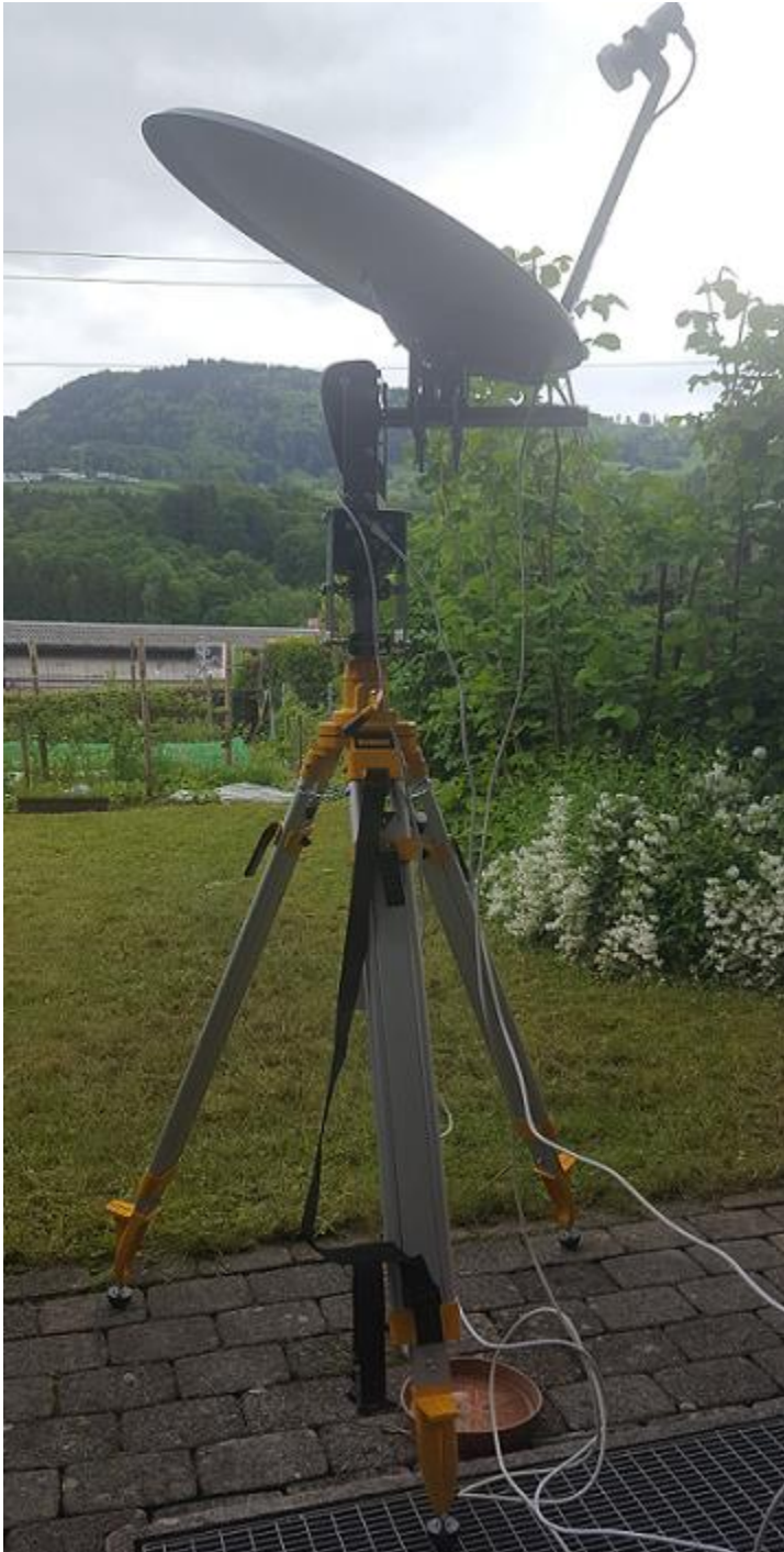
Figure 1 ~ View of the complete telescope (frontend), pointing to the sun. Main components are:
