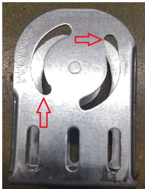
Figures 4a, b ~ Circular slits for antenna mounting need to be extended by about 10 mm, such that the offset angle of the antenna can be fully compensated for. Drill a hole and file it wide enough as depicted in figure 4b (red arrows).
