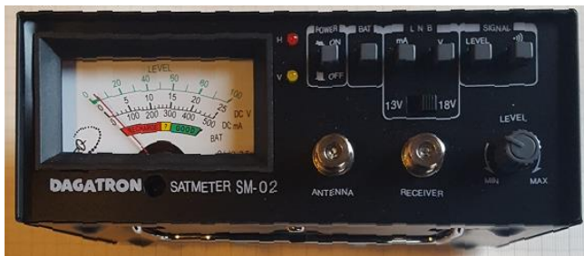
Figure 3 ~ Satellite Finder DAGATRON SATMETER SM-02 from CONRAD works fine down to about 10.6 GHz. Unit is expensive because it also contains a battery and allows control of the LNB. Allows in addition to change polarization and to measure voltage as well as current of the connected LNB.
