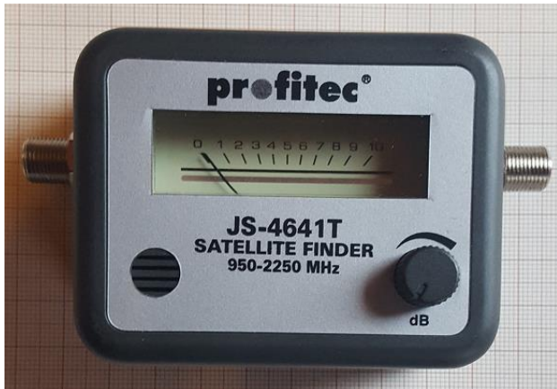
Figure 2 ~ Analogue Satellite Finder Profitec JS-4641T from Amazon with analogue display and beeper works fine for frequencies above about 11.15 GHz. But not usable below that frequency due to high attenuation. Button dB allows to change sensitivity of display and beeper.
