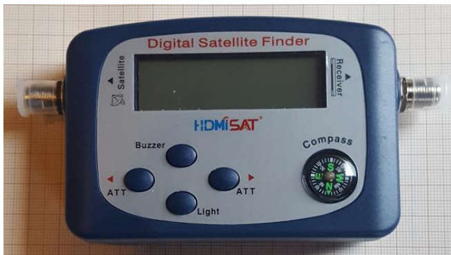
Figure 4 ~ Digital Satellite Finder HDMiSAT SF-9509C from Amazon with internal amplifier and attenuator. Compass bottom right can be used to roughly set azimuth direction of the telescope.
