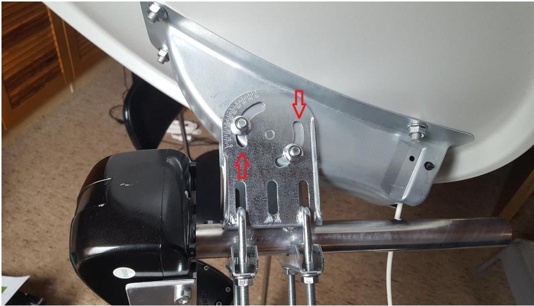
Figure 2 ~ Detail of dish mounting on the elevation axis. Red arrows show slits and bolts to adjust dish-offset in a way, that incoming radiation is perpendicular to the elevation axis. Depending on manufacturer the slits might be extended with a rasp or milling cutter. In this example the dish must be rotated further anti-clockwise to meet the goal. In addition the clamp needs to be rotated by 180° due to the position of the slits.
