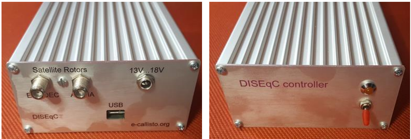
Figure 7 ~ DiSEqC control unit. Left: backside with F-connector for two satellite rotors and USB-connector. Right image: Front panel with LED and power switch.
