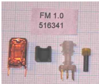
Figure 2: FM1.0 parts from left-to-right: metal-can, ferrite jacket, coil form, ferrite core (yellow). (courtesy of Christian Monstein)
