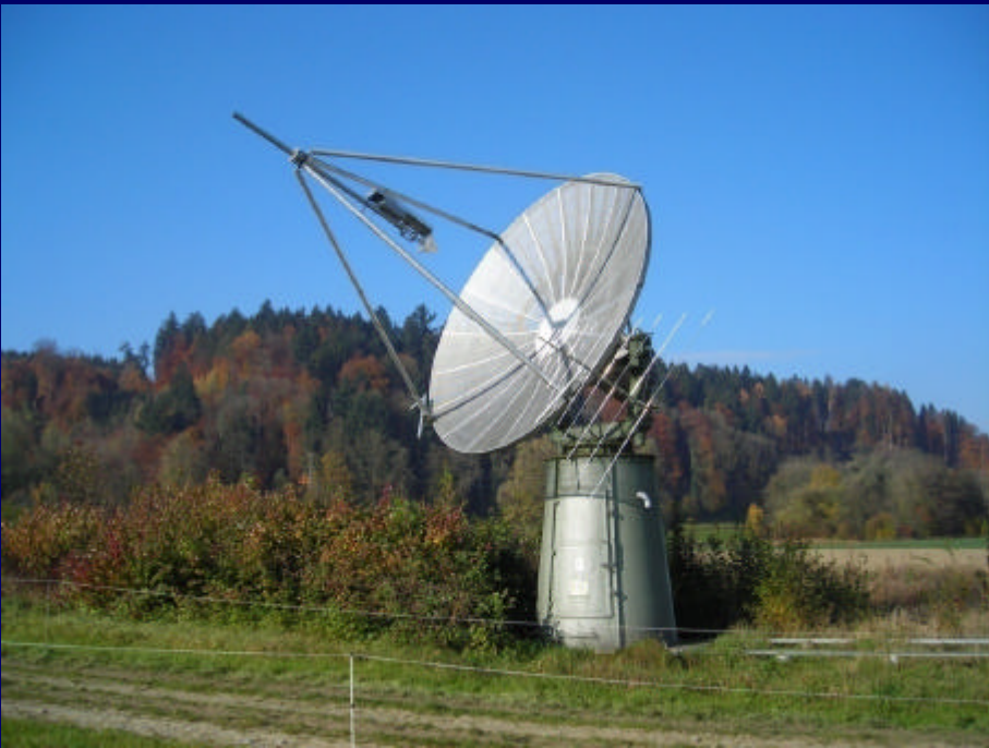
5m parabolic antenna with feed 1GHz - 5GHz
