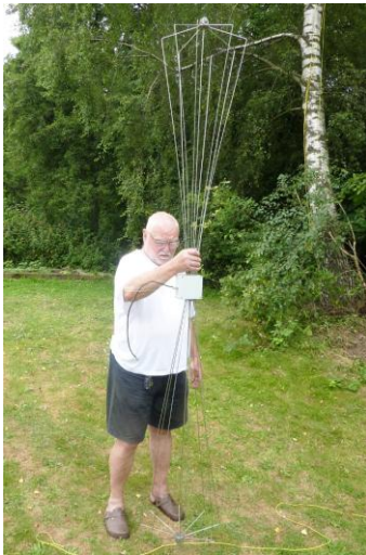
Figure 1 ~ The biconical antenna and the responsible engineer Hannes during installation
