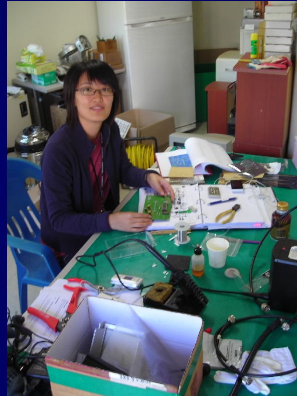
Student Hee-Sun reproducing a Callisto-spectrometer as a semester work in physics.
