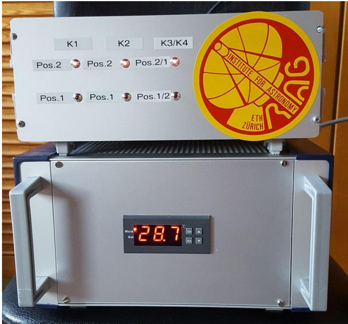
Fig. 1: Top: Calibration unit containing microwave relays, noise source, attenuators, low noise amplifier and Peltier cooler. Bottom: Control unit contains power supply for electronics, low noise amplifier and 28 volts supply for noise source as well as 28 volts for microwave relays. Display below shows current temperature ( ^{\circ}\text{C} ) of the calibration source which has to be taken into account for the evaluation of noise temperature. Control unit allows to keep temperature constant, based on Peltier cooler.
